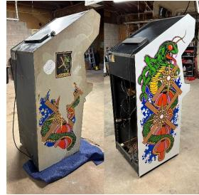
help of my wife Mindy we were able to get it applied. Before that though, I smoothed out the sides/front of the machine by using bondo (auto body filler) and lots of sanding. So after repairing the monitor, the control panel, the power supply, the PCB, and the cabinet itself...the game is now ready to play! ~Ross Aho
